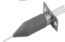
A 1550 nm MQW-DFB InGaAsP laser diode pigtail-coupled to a fiber. (Courtesy of Alcatel.)
