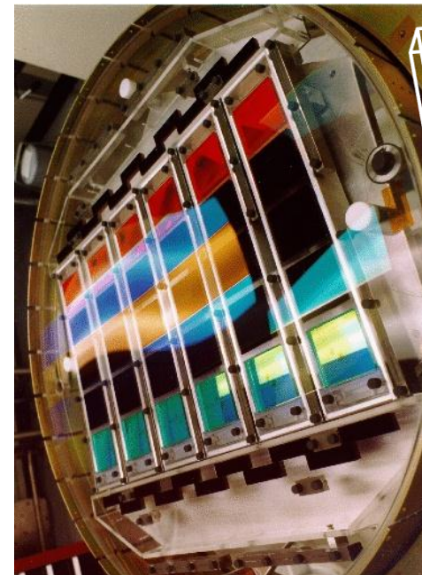
Array of 30 CCDs used on Sloan Digital Sky Survey telescope imaging camera
